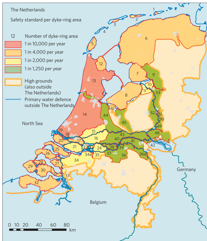
Figure 1 | Flood safety standards of dykes in The Netherlands. The current level of protection ranges from a flooding probability of 1 in 1,250 per year inland to 1 in 10,000 per year along the coast.
