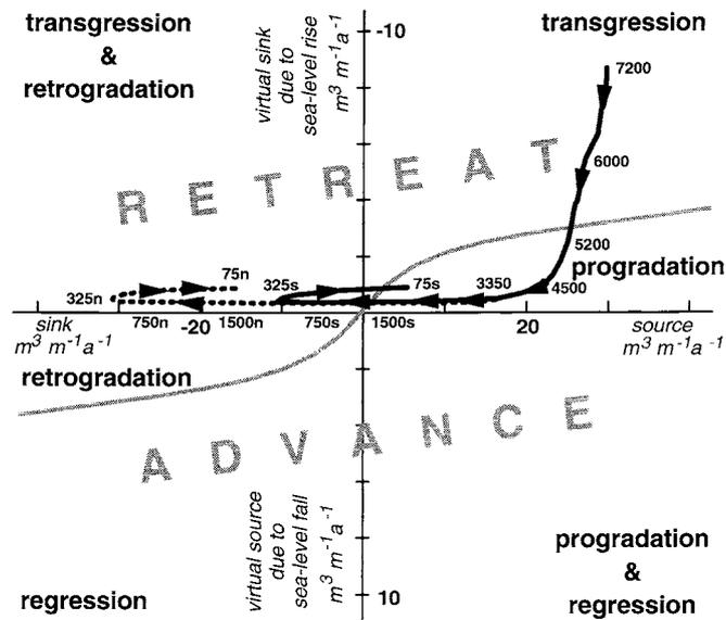
Figure 1. Evolution of the central Netherlands coast (Hoek of Holland to Den Helder) as a time trajectory in sediment-supply/accommodation phase space (abscissa and ordinate respectively, scaled in cubic meters per year per meter of shoreline). Numbers along the trajectory indicate time (years BP); suffixes n and s denote north and south of Haarlem respectively (after Cowell et al., 2003a).
