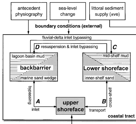
Figure 3. Schematic representation of mechanisms steering the location of the upper shoreface (after Cowell et al., 2003b).
